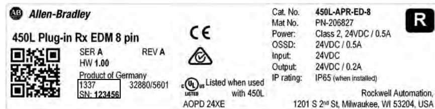
Figure 45 - Explanation of Date Code at a 450L Plug-in [1337: Year 2013, Week: 37; Serial Number Is 123456]
