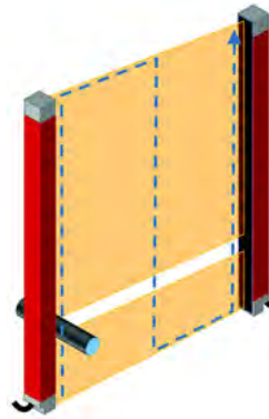
Figure 43 - Proper Testing of Protective Field Using Test Rod
