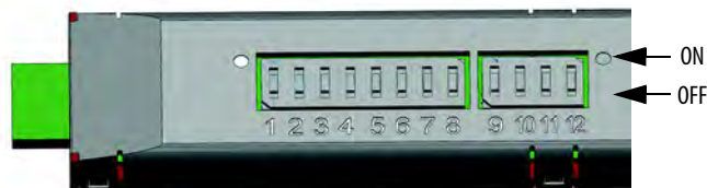
Figure 8 - DIP Switch Location at Receiver Plug-in (Number of DIP Switches Varies Depending on Plug-in Type)
