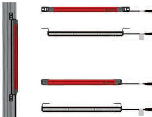
Figure 28 - 450L-B GuardShield Mounted Backwards on an Extruded Aluminum Profile Using the Standard Top/Bottom Mounting Bracket
